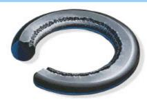
Description: The seal often exhibits discoloration, as well as powdered residue on the surface and possible erosion of elastomer in the exposed areas.
