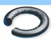
Description: The seal may exhibit radial cracks located on the highest temperature surfaces. In addition, certain elastomers may exhibit signs of softening—a shiny surface as a result of excessive temperatures.
