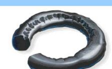
Description: The seal may exhibit many signs of degradation including blisters, cracks, voids or discoloration. In some cases, the degradation is observable only by measurement of physical
