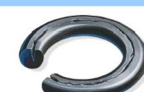
Description: The seal exhibits parallel flat surfaces (corresponding to the contact areas) and may develop circumferential splits within the flattened surfaces.
