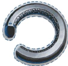
**Description:** This failure is often very difficult to detect from examination of the seal. The seal may exhibit a decrease in cross-sectional size.
