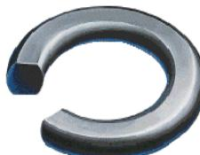
**Contributing Factors:** Excessive compression. Excessive temperature. Incompletely cured elastomer. Elastomer with high compression set. Excessive volume swell in chemical.
