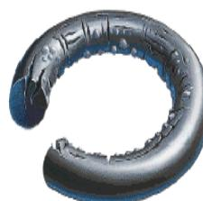
**Contributing Factors:** Rapid pressure changes. Low-modulus/hardness elastomer.
