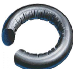
**Description:** The seal may exhibit radial cracks located on the highest temperature surfaces. In addition, certain elastomers may exhibit signs of softening—a shiny surface as a result of excessive temperatures.
