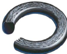
**Contributing Factors:** Rough sealing surfaces. Excessive temperature. Process environment containing abrasive particles. Dynamic motion. Poor elastomer surface finish.
