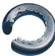
**Contributing Factors:** Excessive clearances. Excessive pressure. Low-modulus/hardness elastomer. Excessive gland fill. Irregular clearance gaps. Sharp gland edges. Improper sizing.
