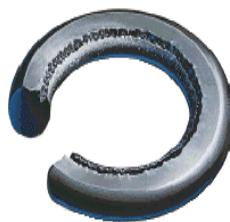
**Description:** The seal often exhibits discoloration, as well as powdered residue on the surface and possible erosion of elastomer in the exposed areas.
