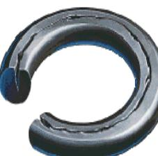
**Description:** The seal exhibits parallel flat surfaces (corresponding to the contact areas) and may develop circumferential splits within the flattened surfaces.
