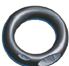
**Contributing Factors:** Sharp edges on glands or components. Improper sizing of elastomer. Low-modulus/hardness elastomer. Elastomer surface contamination.
